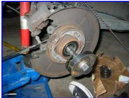
Install a new snap ring. I'm sure you can reuse the old one but a new one is under \$4.00 at the parts counter. If the snap ring will not fit into the groove, the bearing is not fully seated. break out the bearing tool again and push it all the way in.
