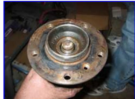
Check the fit of the hub on the stub axle. You should be able to push the hub on far enough to expose enough threads to get the axle nut started.
