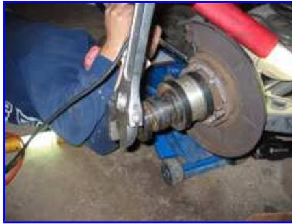
Remove the snap ring holding the bearing in (not shown). Assemble your bearing tool.
