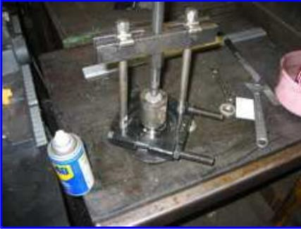
The inner bearing race usually stays with the flange as you pound it out. Use a bearing separator or a 3 leg puller to remove the race. (E30 hub shown)
