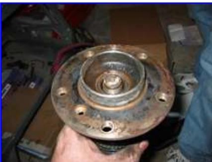
If you have to pound the axle into the hub, you run the risk of pushing the outboard inner race
