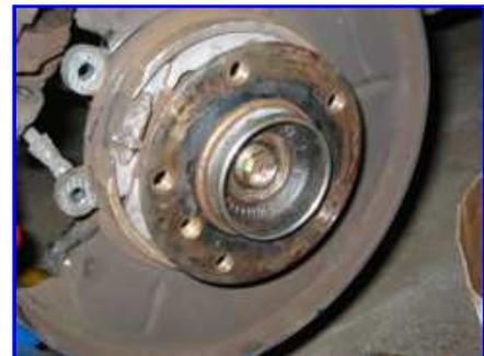
Slide the axle into the hub. Thread the new axle nut on a couple turns
