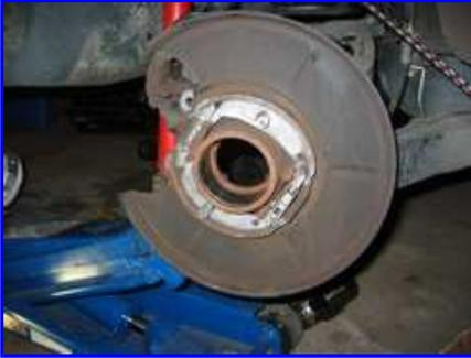
The bearing is out! Clean everything with your favorite solvent and wipe clean. The new bearing should be installed dry. use the largest mandrel possible on the outboard side to push on as much of the bearing outer race as possible. Pushing on the inner race can damage the bearing.
