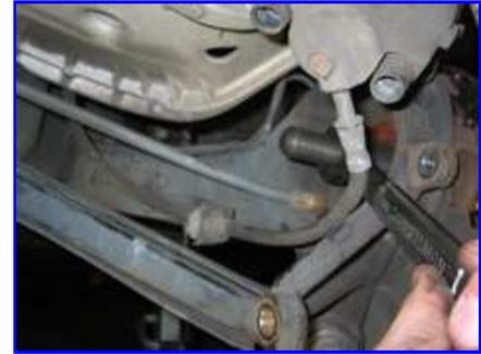
Use the largest mandrel possible that will clear the control arm on the inboard side of the bearing. You want to push on as much area of the bearing as possible to avoid pushing out just the inner races.
