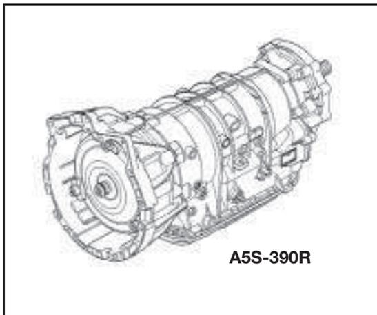
The automatic transmission for both the 330xi and 325xi is the A5S-390 R (General Motors) transmission with GS 20 AGS control and Steptronic shifter.
