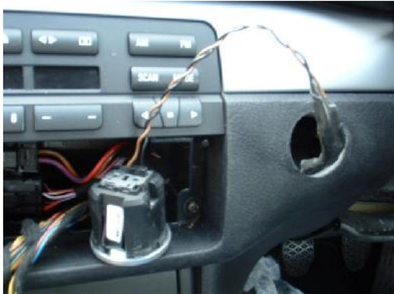
Nearly done now. Vacuum or dust out all plastic cuttings that are around the dash and carpets after the hole was drilled. Push back in the climate display and refit the panel around the pedals, don't forget to refit the clutch pedal stop. Refit the driver's glove box and you're finished. ENJOY!
