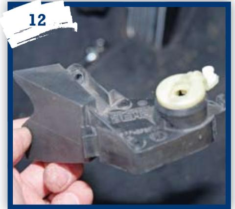
12 The housing is held by two Torx screws – the lower one you can see, but the upper one is almost impossible to see with your head under the dash, so this shot of the part out of the car shows what you're looking at. You'll need a slim Torx bit to fit inside the moulded gallery for the screw but it will also need to be short enough to clear the steering column. If you're lucky, you can catch it with a small flat-bladed screwdriver but be careful not to round the head off.
