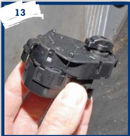
13 The stepper motor itself is simply unclipped from the housing by squeezing the retaining clips which are moulded into its body.
