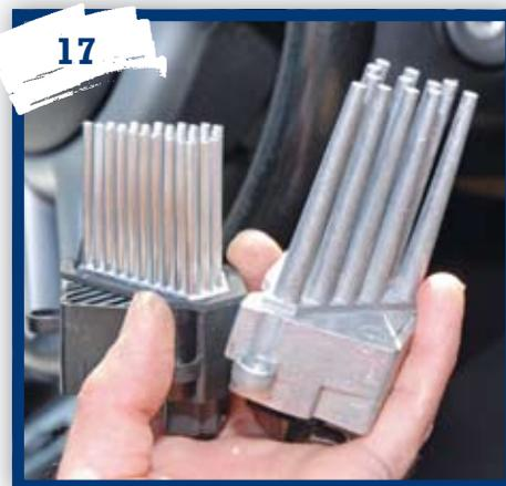
17 Here you can see the old and new resistors compared, with the new unit from Motormec on the left. Don't worry if they don't look identical as BMW itself went through three designs on the E46 alone. Refitting it is as they say in the best books, the reverse of removal but make sure you seat the new resistor firmly enough for the retaining clip to engage securely.
