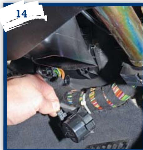
14 The control linkage can also be unclipped to allow the housing to be removed completely.
