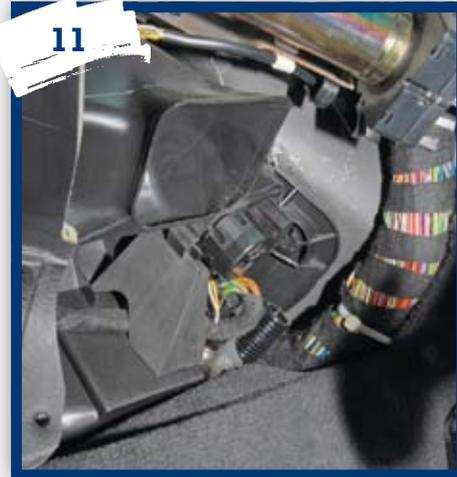
11 With the trim panel out of the way, you can see the resistor – or at least the general area where it lives. It's partially hidden behind the plastic moulding which houses one of the stepper motors for the air conditioning, and you'll need to remove this before you can slide out the resistor.
