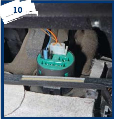
10 ... while the wiring for the warning buzzer simply unplugs. Remember to disconnect the courtesy light for the footwell and you're done.
