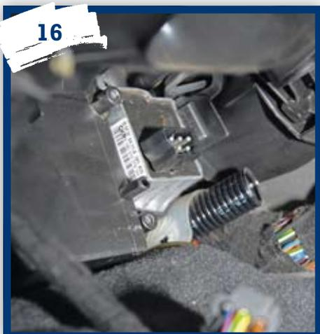
16 Simply unplug the wiring connector and then ease the retaining clip to one side and slide the resistor out. We found the clip was hard work and the resistor needed a fair bit of wiggling after being in there for nine years.
