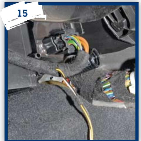
15 With that lot out of the way, the resistor is revealed.
